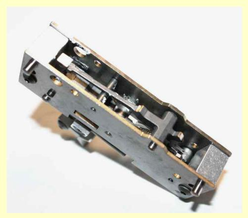
Clean the trigger mechanism with the same Bake Cleaner and air dry VERY WELL. Repeat. You can not dry it too much.
