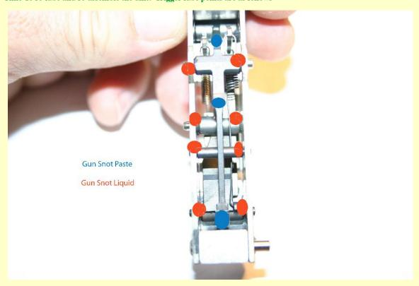
Notice that we use way more Gun Snot... Liquid Lube than Gun Snot Paste Lube. There are 8 Gun Snot Liquid Lube points on top and 3 Gun Snot Paste Lube points. The 'stiction' of the Gun Snot Paste Lube is too high for most parts in the trigger, but they are supreb for high load points. We do add Gun Snot Paste Lube to the sear and contact points. Basically you <u>lubricate anything that moves or is shiny</u>. From the bottom look for points of movement or shine and use Gun Snot Liquid Lube only.
