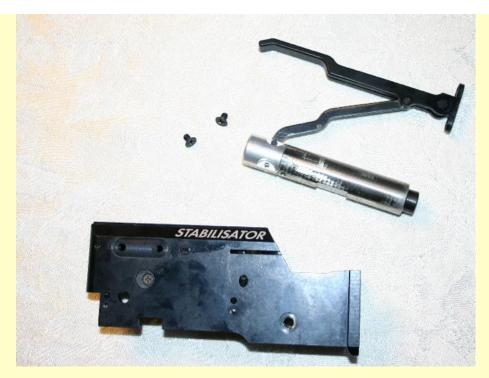
Now you want to remove the trigger housing from the breach. Firstly there is a cocking plate (133) that has to come off. Try and pay attention to how it comes out, as there is a trick to getting it back together and it all rests in that piece. There are 3 screws (65) that need to removed to lift this plate out.
