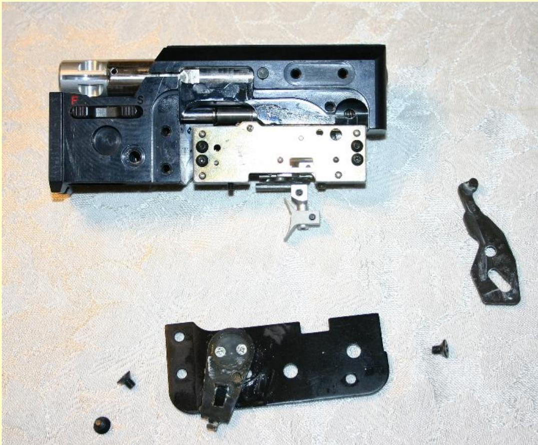
The next step is to remove the bolt (92) from the breach. The bolt is chrome and there is a stabilizer [spring loaded cylinder] (200, 201, 202, 203, 204, 205) behind it. It is critical to note the orientation of the bolt so that its holes line up with the sear and lever cocking plate (106) and bolt (103) later.
