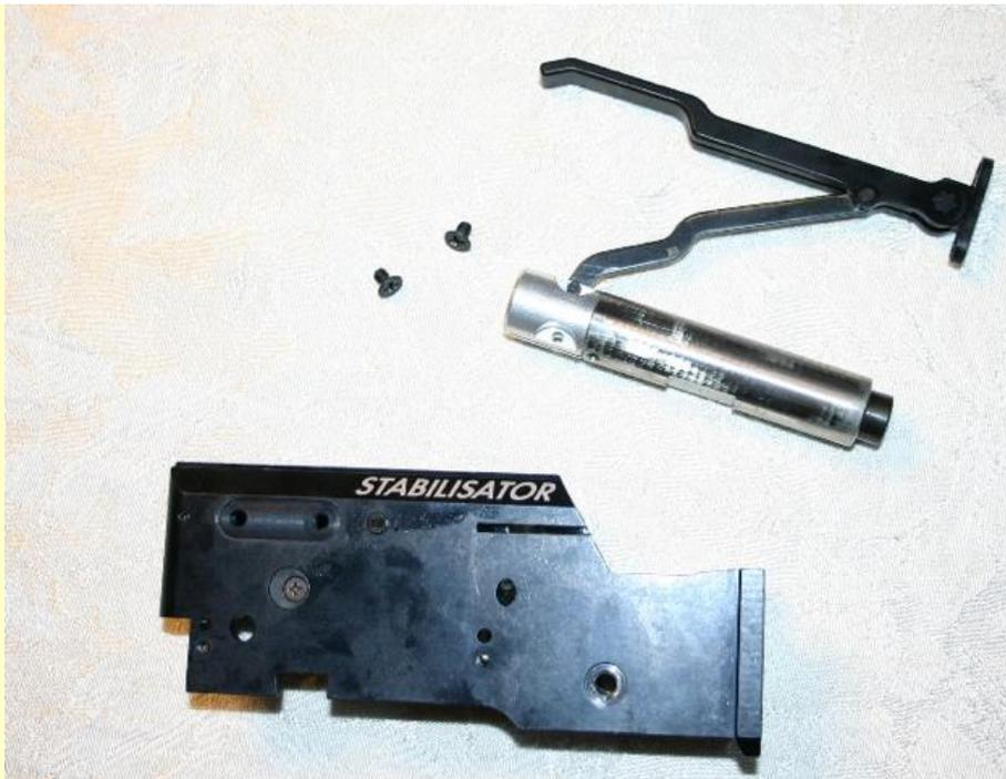
Now you want to remove the trigger housing from the breach. Firstly there is a cocking plate (133) that has to come off. Try and pay attention to how it comes out, as there is a trick to getting it back together and it all rests in that piece. There are 3 screws (65) that need to be removed to lift this plate out.
