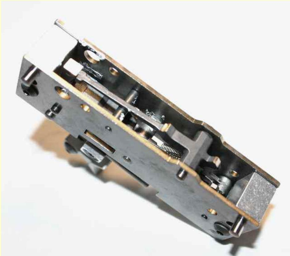
Clean the trigger mechanism with the same Brake Cleaner and air dry **VERY WELL**. Repeat. You can not dry it too much.
